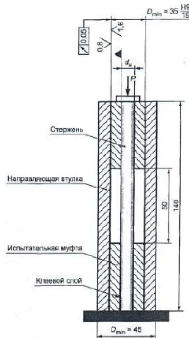
Figure B.2. – Compression Test Device of Samples
